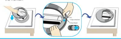
■ Tighten the four □ screws about half into the slots in the base part, hold the two screws at the bottom to pull them inward, and then tighten the screws all the way.
