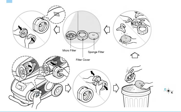
The dust filter is located below the filter cover as in above figure. If the LED is lighted up when the dust tank is not full, firstly clean the air filter.
