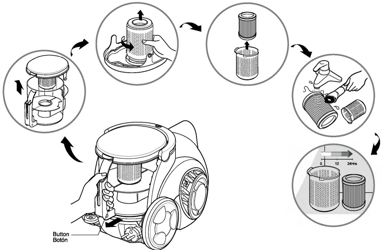
The reusable filters are situated under the dust chamber cap and you can use it permanently.
