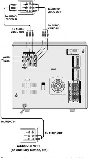
Connect a VCR or auxiliary device, etc to the AUX 1 connector.
