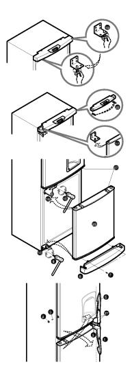
6. Stop the groom where the existing HANDLE ①, ③ was installed at by using the CAP ④ removed in the initial installation.
