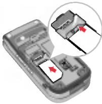
To insert the USIM card
