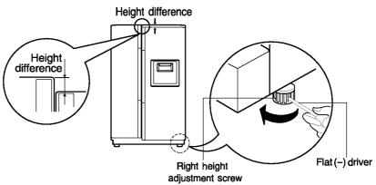
The refrigerator doors will close smoothly by heightening the front side by adjusting the height adjusting screw. If the doors do not close correctly, performance may be affected.
