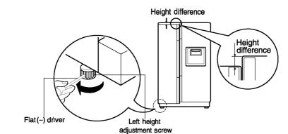
Level the door by inserting flat (- type) driver into the groove of the right height adjusting screw and rotate it to the arrow direction ( $_{\downarrow}$ ).
