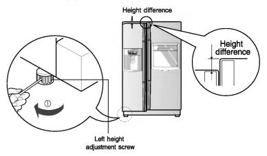
If the freezer compartment door is higher than the refrigerator compartment door Level the door by inserting flat ( - type) driver into the groove of the right height adjusting screw and rotate it clockwise  $(\mathbb{O})$ .
