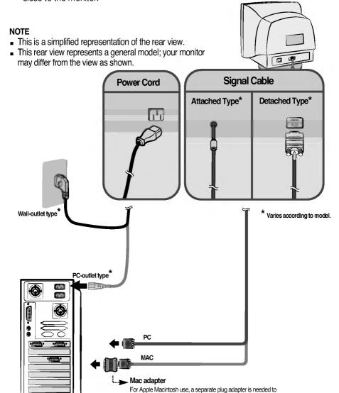
change the 15 pin high density (3 row) D-sub VGA connector on the supplied cable to a 15 pin 2 row connector.
