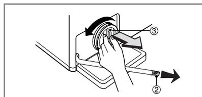
2. Unplug the drain plug (2), allowing the water to flow out. At this time use a vessel to prevent water flowing on to the floor. When water does not flow any more, turn the pump filter (3) open to the left.
