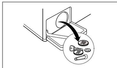
3. Remove out any foreign material from the pump filter.
