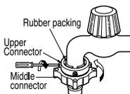
3. Connect the water supply hose to the middle connector, pushing the plate down.
