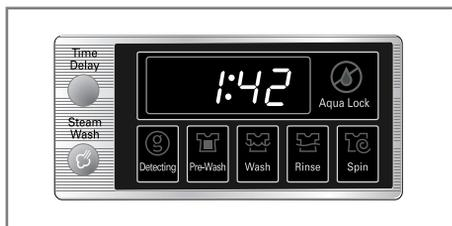
By pressing the Steam Wash button, Steam Function Can be selected.
