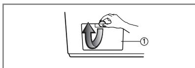
1. Open the lower cover cap (1) by using a coin.
