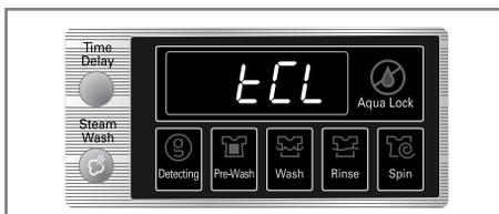
**TUB CLEAN** is special cycle to clean the inside of the washer. This cycle uses higher water level with higher spin speed. Perform this cycle regularly.
