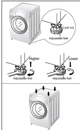
2. If the floor is uneven, adjust the adjustable feet as required.
