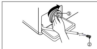
4. After cleaning, turn the pump filter (3) clockwise and insert the drain plug (2) to the original place. Close the lower cover cap.
