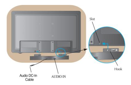
3. After setting up the speaker, connect the Audio DC-In Cable to the back of the product.
