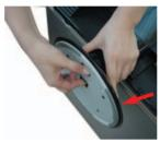
**4.** Separate the stand using a screwdriver as shown in the picture. **Note:** Please keep the 4 screws in an accessible place for future use.
