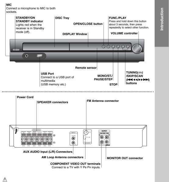
Do not touch the inner pins of the jacks on the rear panel. Electrostatic discharge may cause permanent damage to the unit.
