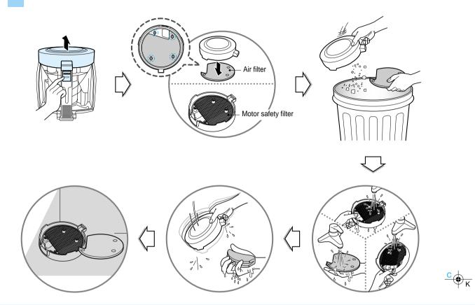
If the indicator is lighted on after cleaning the dust tank, clean the air filter and motor safety filter. The air filter and motor safety filter are located at the bottom of dust tank cap in above figure.
