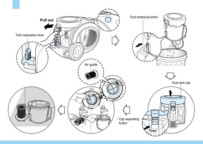
Check the indicator is lighted on after emptying the dust tank. If the indicator is lighted on when dust tank is not filled, firstly clean the dust tank and air guide as follows.
