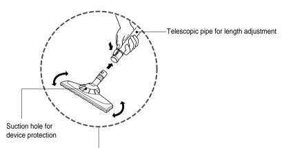
You can perform cleaning at any place like corner or crevice since revolution of the suction hole is free.
