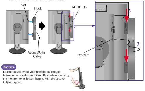
**4.** Connect the audio cable to the AUDIO-IN terminal. When using HDMI, you can connect the monitor's to the AUDIO-OUT terminal. When using a PC or other component, simply connect to the appropriate female socket of the external instrument.
