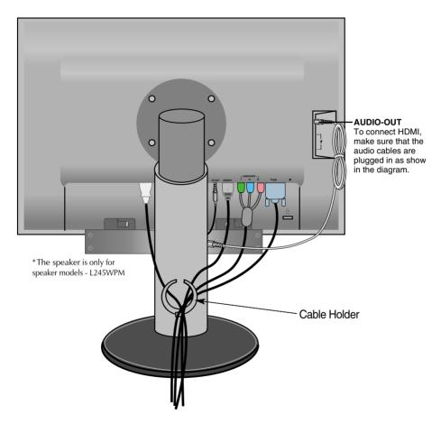
\*The length of the cable which connects the monitor's AUDIO-OUT and the speaker's AUDIO-IN can be too long. It is used to connect the components at the appropriate distance when the AUDIO-IN terminal and the speaker are connected to the PC.
