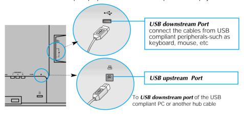
3. The monitor's USB terminal supports USB 2.0 and High Speed cables.
