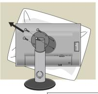
**2.** Separate the head and the stand with the use of a screwdriver.
