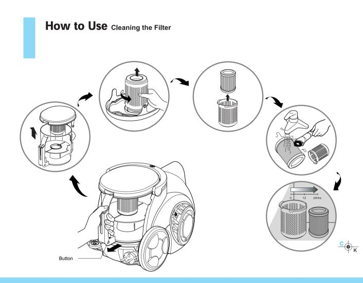
The reusable filters are situated under the dust chamber cap and you can use it permanently.
