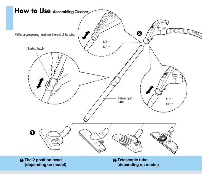
Push telescopic tube into nozzle outlet.
