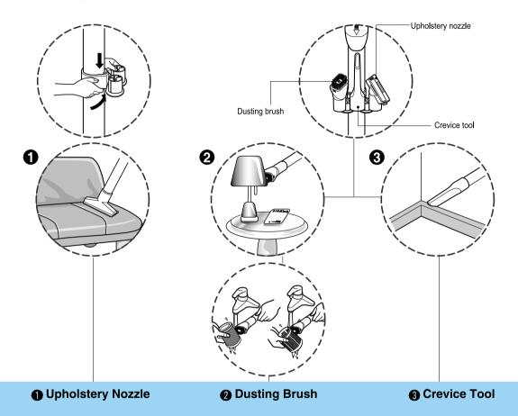
Upholstery Nozzle is for vacuuming upholstery, mattresses, etc. The thread collectors help to pick up the threads and fluff. Dusting Brush is for vacuuming picture frames, furniture frames, books and other irregular surfaces. Dusting Brush is also used for cleaning Filters. Crevice Tool is for vacuuming in those normally hard-to-reach places such as reaching cobwebs, or between the cushions of a sofa.
