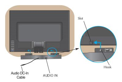
${f 3.}$  After setting up the speaker, connect the Audio DC-In Cable to the back of the product.
