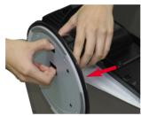
**4.** Separate the stand using a screwdriver as shown in the picture. **Note:** Please keep the 4 screw in an accessible place for future use.
