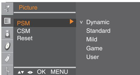
The **PSM** function automatically adjusts the screen image quality.
