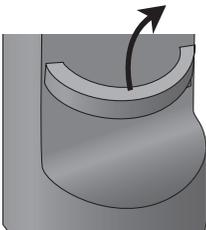
Hold the cable management and lift up slightly to remove it.
