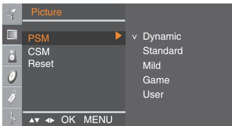
The **PSM** function automatically adjusts the screen image quality. (It is not working in PC input.)
