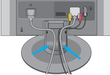
2. Fit the cable management to the Holder Groove downwards.
