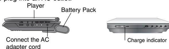
3. During recharging, charge indicator is red. If recharging is complete, charge indicator changes to green color.
