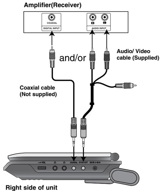
**Amplifier equipped with 2-channel analog stereo or Dolby Pro Logic II / Pro Logic:** Connect the AV IN/OUT jacks on the unit to the audio left and right IN jacks on your amplifier, receiver, or stereo system, using the audio cables.
