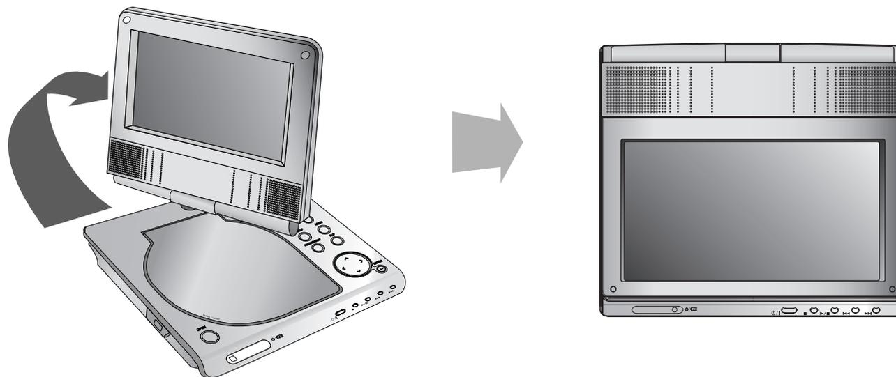
You can rotate LCD clockwise an angle of 180 degrees. However, if you turn it by force, it can cause serious damage.
