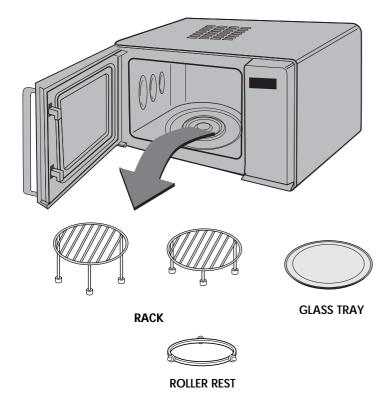
Place the oven in the level location of your choice with more than 85cm height but make sure there is at least 30cm of space on the top and 10cm at the rear for proper ventilation. The front of the oven should be at least 8cm from the edge of the surface to prevent tipping.
