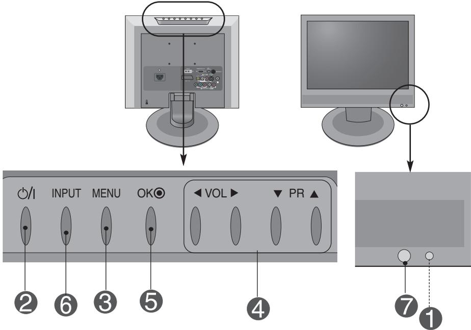
**1** **Power Indicator** • This Indicator lights up green when the display operates normally (On Mode). If the display is in Sleep (Energy Saving) Mode, this indicator colour changes to red.
