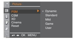
The **PSM** function automatically adjusts the screen image quality.
