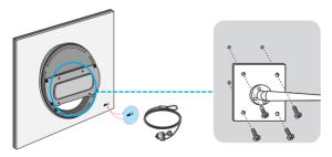
Kensington Security Slot Connected to a locking cable that can be purchased separately at most computer stores
