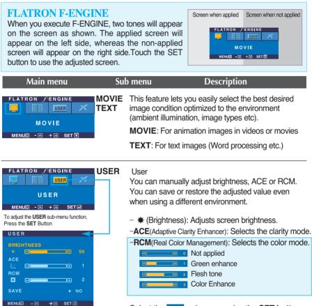
Select the **SAVE** sub-menu using the **SET button** and save the **YES** value using the **buttons**.
