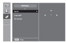
You can assign a unique **Set ID** NO (name assignment) to each product when several products are connected for display. Specify the number (1~99) using the ▲ ▼ button and exit. Use the assigned Set ID to individually control each product using the Product Control Program.
