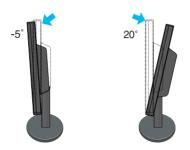
Warning: When adjusting the angle of the screen, do not put your finger(s) in between the head of the monitor and the stand body. You can hurt your finger(s).
