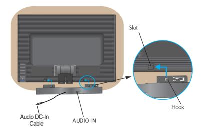
3. After setting up the speaker, connect the Audio DC-In Cable to the back of the product.
