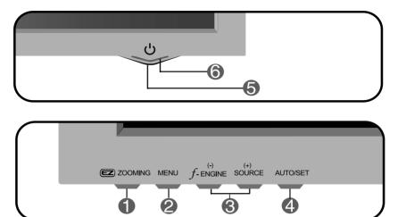
**1 EXAMPLANCE** At the current display, Use 'ez Zooming' Key, then the display resolution is transferred to the one step low resolution. Use 'ez Zooming' Key one more, the display is back to the original display.
