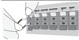
Connect the red end of each wire to the terminals marked +(plus) and the black end to the terminals marked - (minus).
