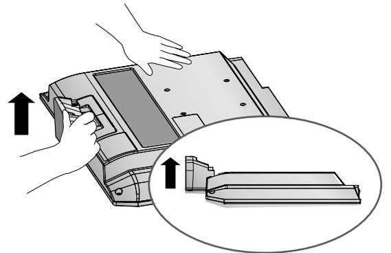
**5** Pull stand body to separate from set during pressing 2 latches.
