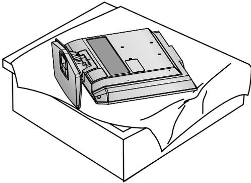
**2** Pull cover base backward during pressing button on stand body.
