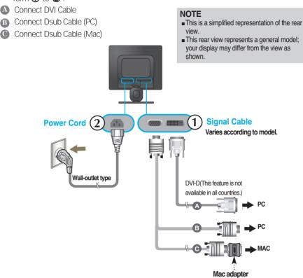
For Apple Macintosh use, a separate plug adapter is needed to change the 15 pin high density (3 row) D-sub VGA connector on the supplied cable to a 15 pin 2 row connector.
