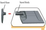
**4.** Insert the Cable Deco Cover in the Stand Body in the correct direction.
