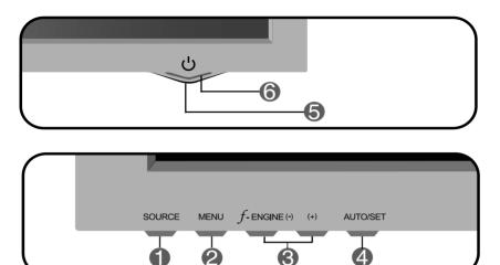
SOURCE ButtonYou can select the computer that you want to use by<br/>selecting input signal (DVI, D-Sub or USB).The default input signal is analogue (D-Sub).
