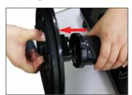
**5.** Slightly pull the stand body to disconnect from the hinge body.
