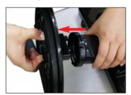
**5.** Slightly pull the stand body to disconnect from the hinge body.
