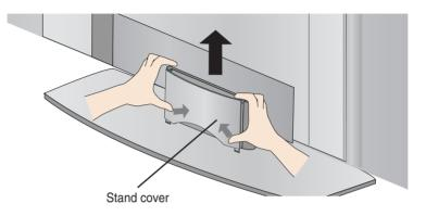
2. After connecting the cables, correctly position the stand cover into the holes on the stand. If securely connected, you will hear the latch click into place.
