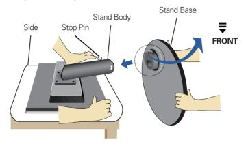
3. Make the monitor stand, then pull out the Stop Pin.
