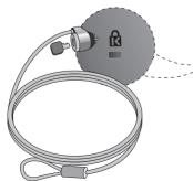
Kensington Security Slot Connected to a locking cable that can be purchased separately at most computer stores
