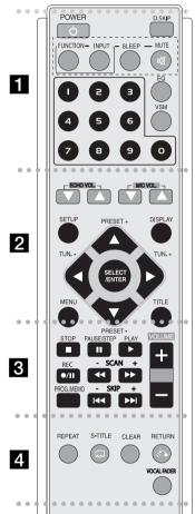
**POWER:** Switches the unit ON or OFF. **DISC SKIP** Choose a desired disc.
