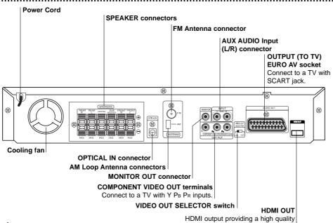
Do not touch the inner pins of the jacks on the rear panel. Electrostatic discharge may cause permanent damage to the unit.
