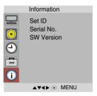
Set ID You can assign a unique Set ID NO (name assignment) to each product when several products are connected for display. Specify the number (1~99) using the ▼ ▲ button and exit. Use the assigned Set ID to individually control each product using the Product Control Program.
