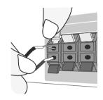
3 Connect the wires to the speakers.
