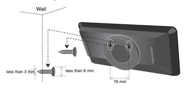
Ensure that the unit locks onto the hooks and that the hooks are strong enough to support the weight before releasing the hand.
