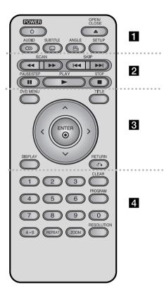
POWER (<sup>()</sup>): Switches the unit ON or OFF.
