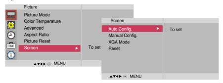
**Auto Config.** (RGB PC input only): This button is for the automatic adjustment of the screen position, clock and phase. This function is available for analog signals only. **Manual Config.**: If the picture isn't clear after auto adjustment and characters are still trembling, adjust the picture phase manually.
