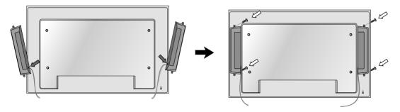
After installing your speakers, use holders and cable ties to organize the speaker cables.
