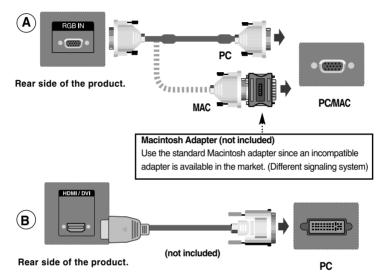
\* User must use shielded signal interface cables (D-sub 15 pin cable, DVI cable) with ferrite cores to maintain standard compliance for the product.
