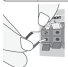
Connect the red end of each wire to the terminals marked +(plus) and the black end to the terminals marked - (minus).
