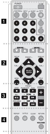
POWER: Switches the unit ON or OFF. DISC SKIP Choose a desired disc.
