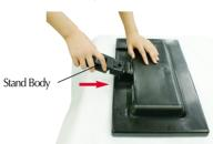
**3.** Assemble the Stand Base into the Stand Body in the correct direction.
