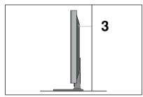
Use a sturdy rope to tie the TV. It is safer to tie the rope so it becomes horizontal between the wall and the TV.
