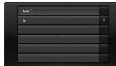
[New ID]: Displays the keyboard menu for entering a new ID and password.
