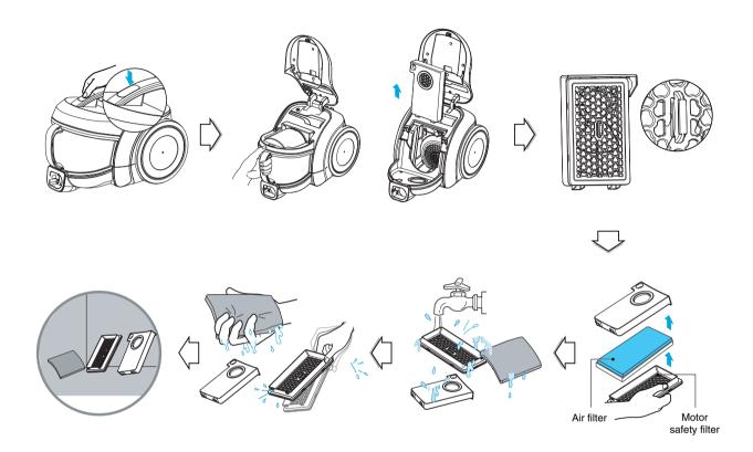
If suction power is decreased after cleaning dust tank, clean air filter and motor safety filter. Air filter and motor safety filter are located at the center of vacuum cleaner in the above figure.
