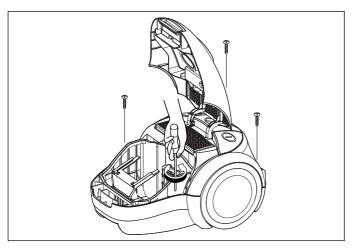
3) Lift body cover assembly in the direction of the arrow.
