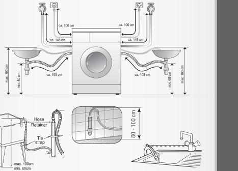
The drain hose should not be placed higher than 100 cm above the floor.
